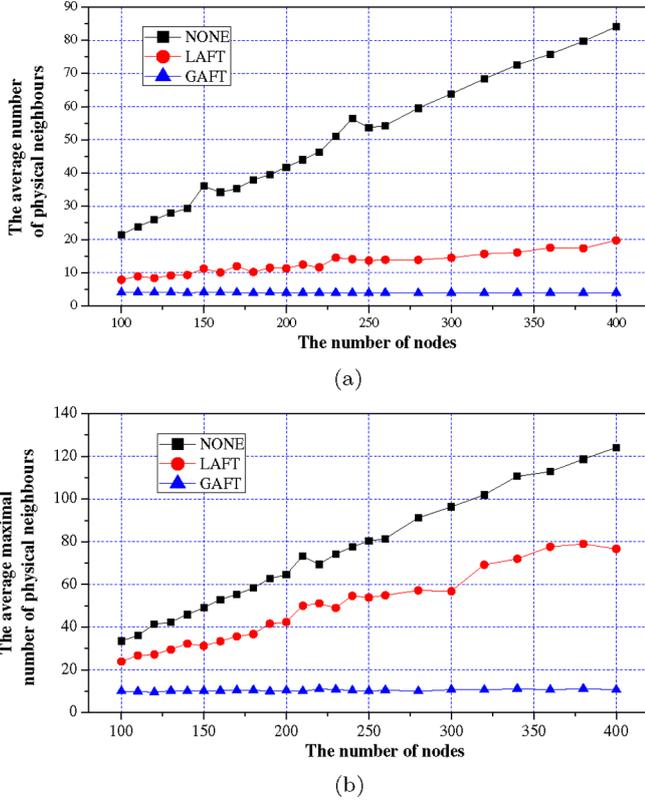
**Figure 6** Comparison of GAFT<sub>k</sub> and LAFT<sub>k</sub> with respect to the physical node degree ( $k = 4$ ): (a) the average number of physical neighbours and (b) the average maximal number of physical neighbours (see online version for colours)
